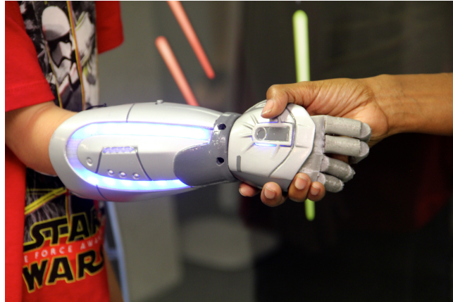
FIGURE 2.6: Prosthetic Arm by Open Bionics (StarWarsRey, 2015). By StarWarsRey, (“CC BY-SA 4.0”, n.d.), via Wikimedia Commons.
